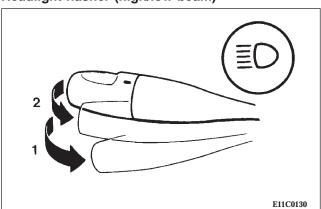
The headlights can be made to flash (high beam) when the lever is pulled slightly to (2), and will go back to normal when it is released. While the high beam is on, a blue light in the instrument cluster will also illuminate.
